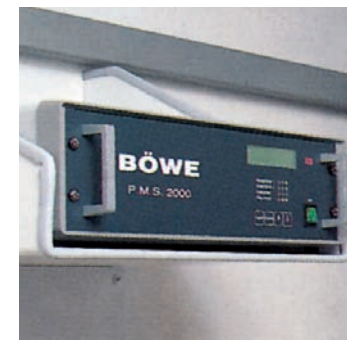
The Perc Measuring System Controls the Residual Solvent Concentration
