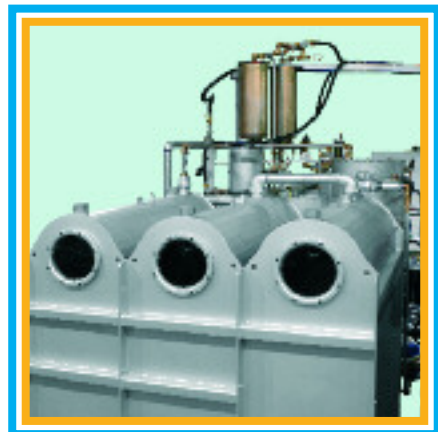
Cleaning of the lint filter - cage housing in loading position
