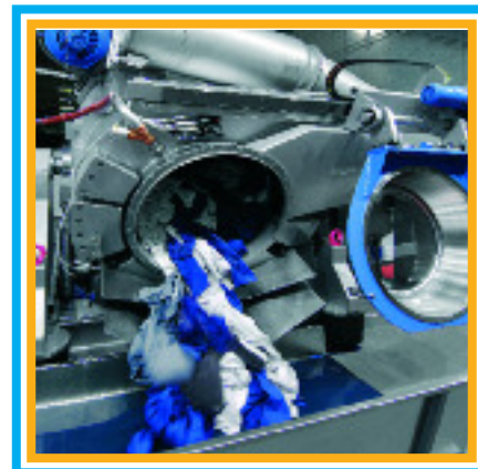
Front view unloading - the cage tilts up to 30° downwards
