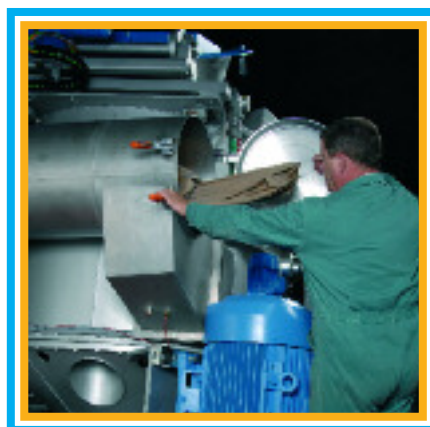
Cleaning of the lint filter - cage housing in loading position
